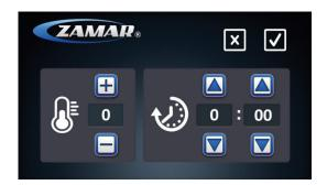
Inside the parameters setting screen you can set the temperature by increasing or decresing with the "+" and "-" keys. The temperature setting can be set within a range of  $+41^{\circ}$ F to  $+59^{\circ}$ F.
