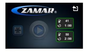
By pressing any button, you will enter in the screen for programming the treatment parameters like temperature and duration of treatment.
