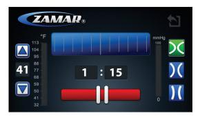
When treatment is executed, the duration parameters starts to count down. The side graduated bar indicates the current temperature of the machine. The horizontal bar above the countdown timer indicates the progress of the treatment.
