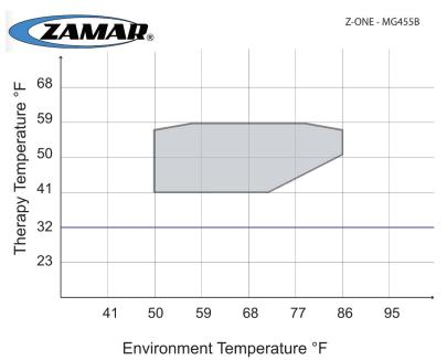
The ambient temperature affects the performance of the device. ZAMAR suggests to remain in a range between 64°F and 75°F in order to make the most of the device.
